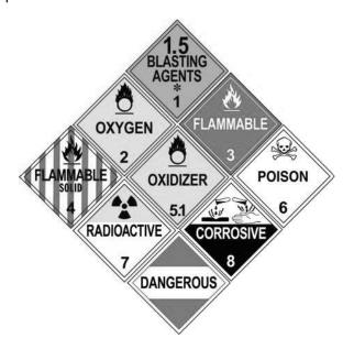
Figure 9.3 - Examples of hazmat placards
