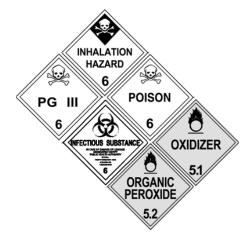
Figure 9.2 - Examples of hazmat labels
